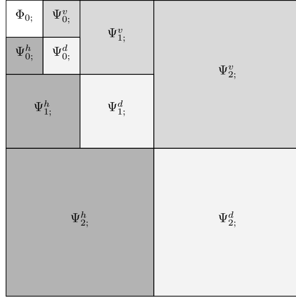
Figure C.10: Non-standard two-dimensional wavelet decomposition. The block labelled \Psi_{2,}^d contains the coefficients of basis functions \Psi_{2,0,0}^d through \Psi_{2,3,3}^d , with a similar convention adopted for the other blocks.
