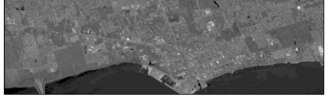
Fig. 1. Broadband image of the 224-channel hyperspectral AVIRIS data used in these experiments. The image is 150×500 pixels, and was obtained from flight f960323t01p02\_r04\_sc01 over the Florida coast.
