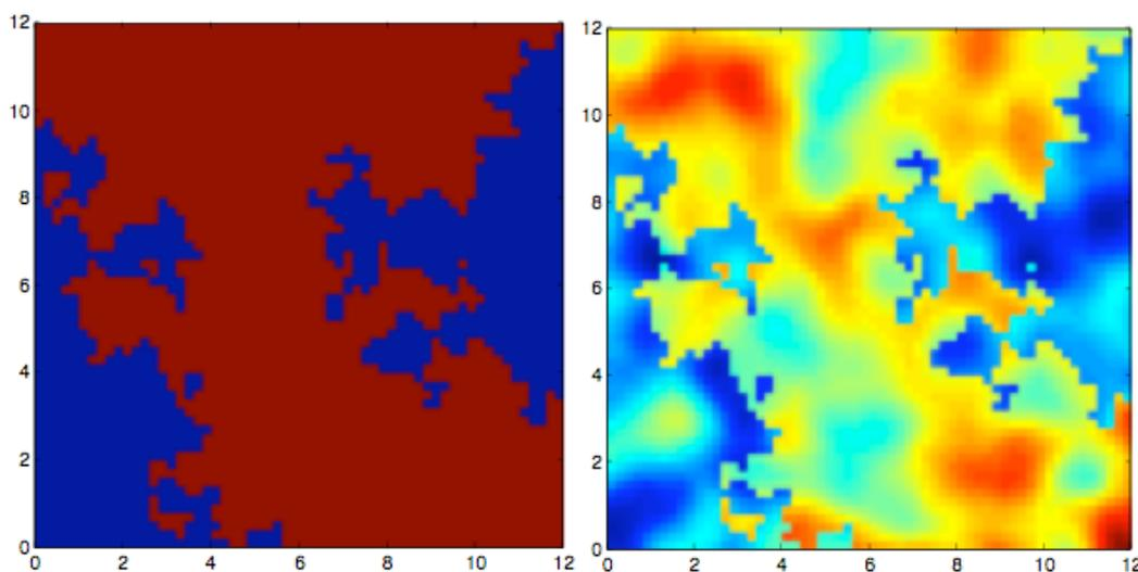
FIGURE 2. (a) Material classification of *Wohlberg et al.* [2006]; and (b) Distribution of log hydraulic conductivity, whose values range from -7.00 (dark blue) to 0.60 (red).
